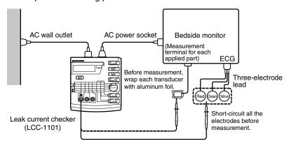
Measure the patient leak current flowing in the measurement system for each parameter. For the ECG, short-circuit all the electrode leads before measurement. For the other parameters, wrap the transducer with aluminum foil before measurement.
