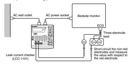
For the ECG, measure the patient measurement current (AC). Short-circuit the non-red electrode leads for the ECG and measure the value with respect to the red one.
