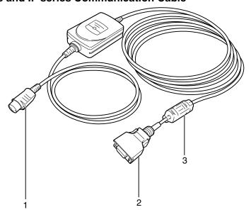
1 Multi-link connector Connect to the multi-link socket on the bedside monitor.
